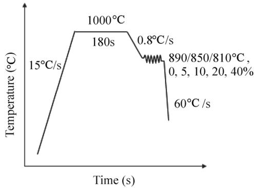
**Fig.1.** The thermal process route for the simulated thermo-mechanical treatment.
