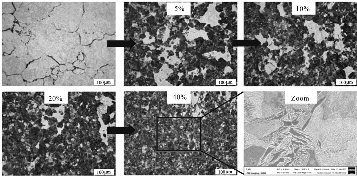
Fig.6. The metallographic images of different deformation strains at 810°C.
