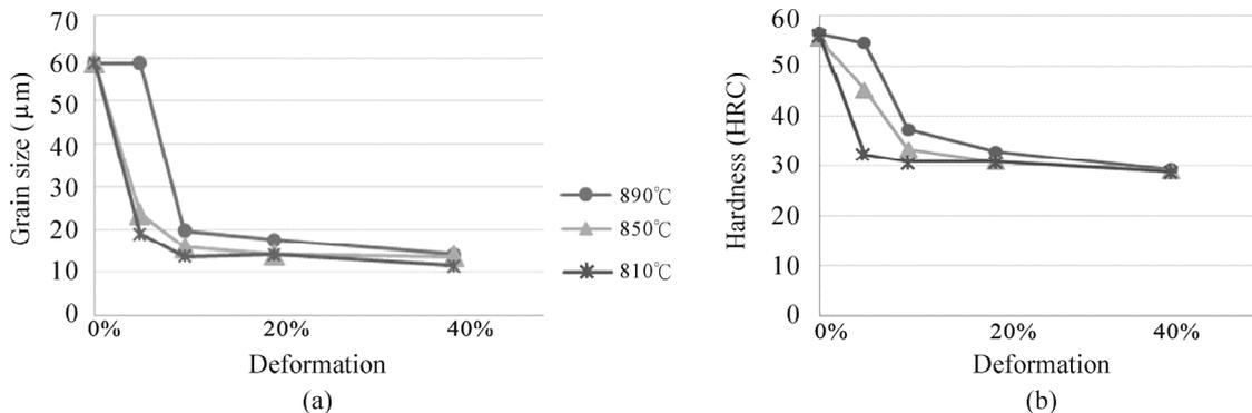
Fig.8. The summary of the experimental results: (a) grain size, (b) hardness vs. deformation strain.
