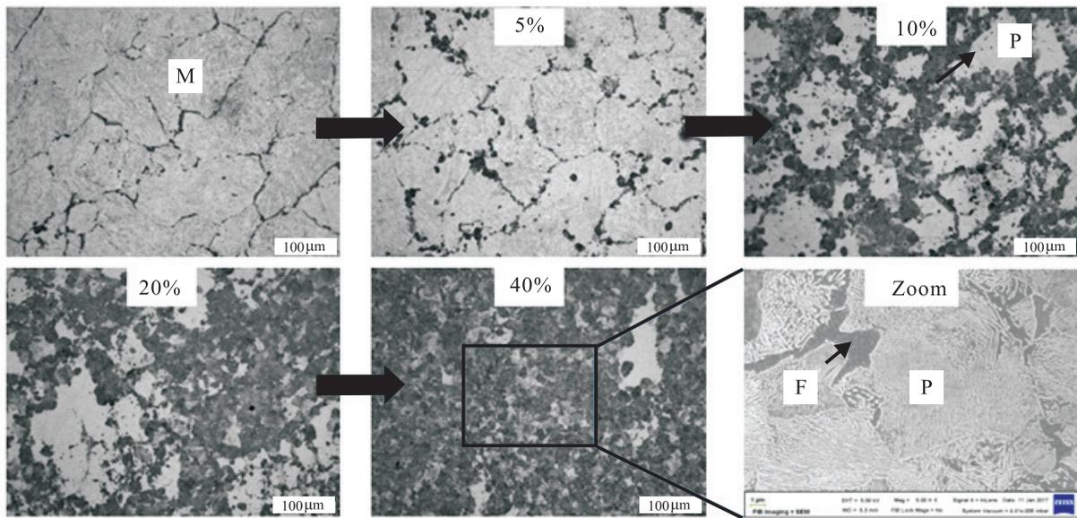
**Fig.4.** The metallographic images of different deformation strains at 890°C. In this images, phases were identified by M (martensite), P (pearlite) and F (ferrite), respectively.
