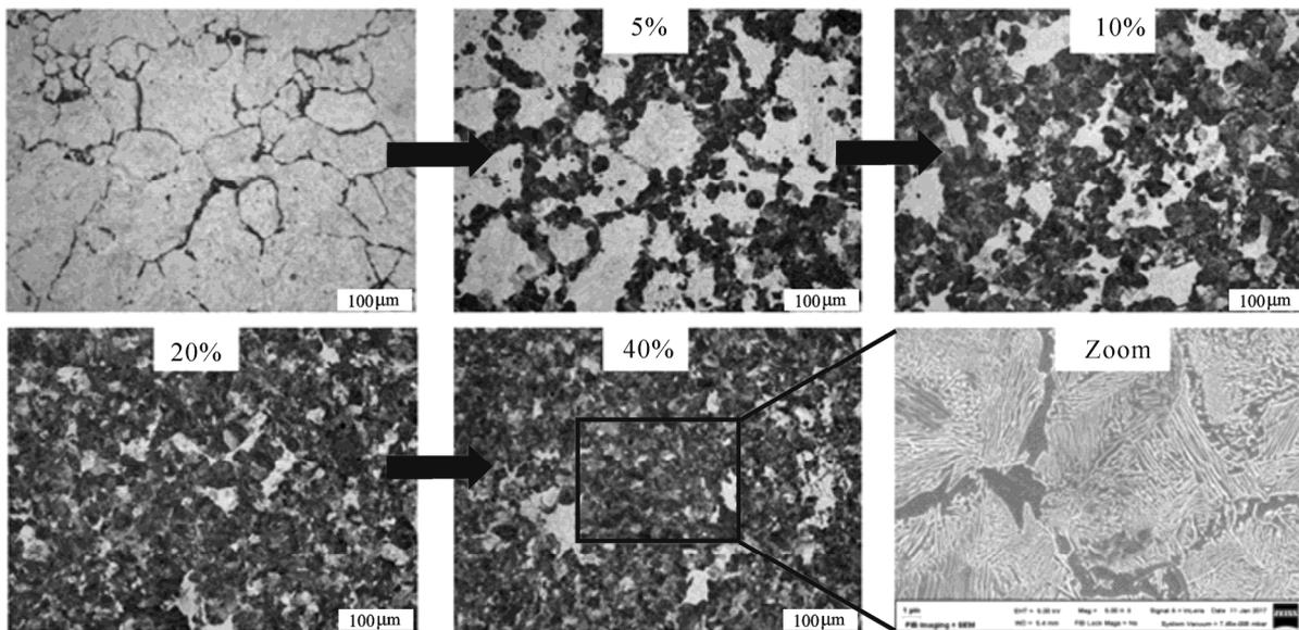
**Fig.5.** The metallographic images of different deformation strains at 850°C.
