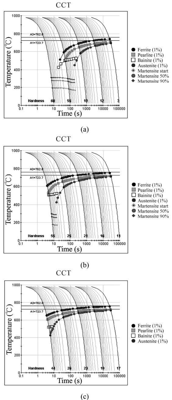
**Fig.2.** The computer-aided steel simulation results of (a) no deformation strain, (b) low deformation strain, and (c) high deformation strain.
