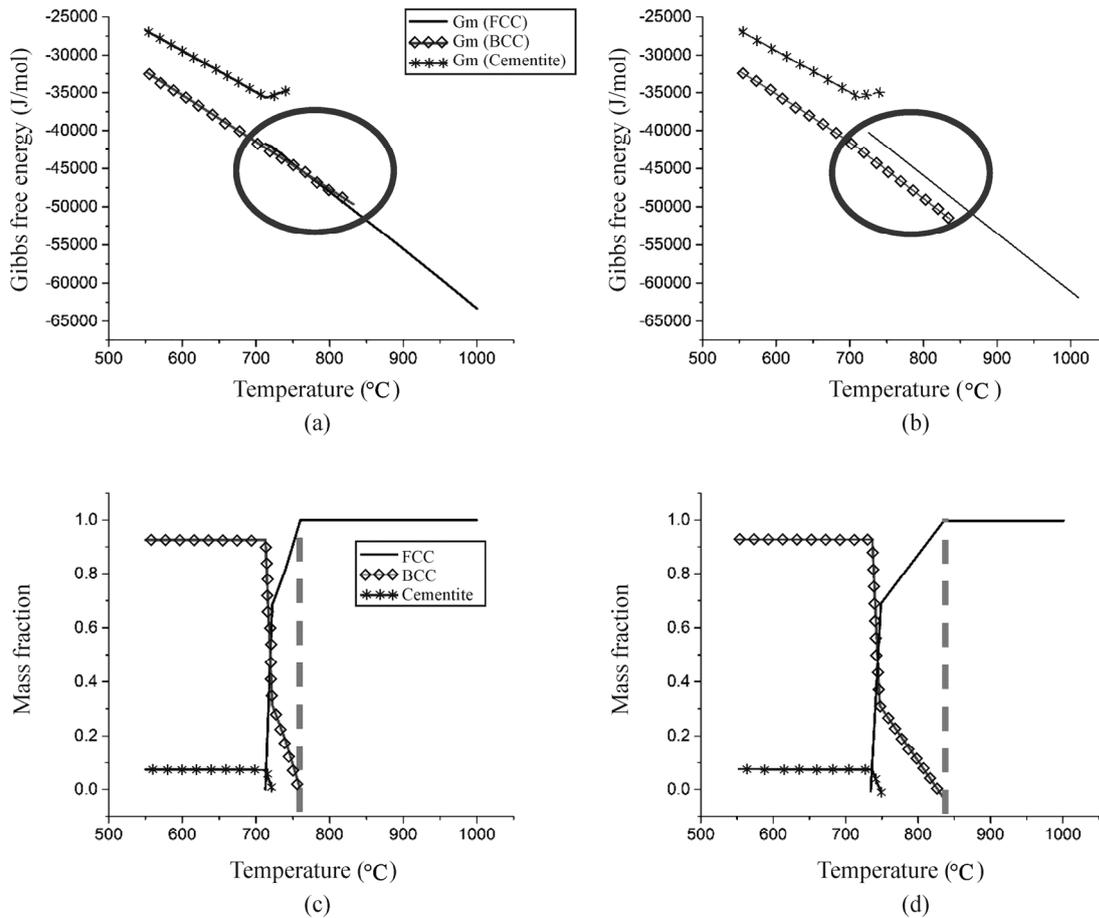
**Fig.3.** The calculation results of the Gibbs free energy and mass fraction of (a) and (c) without and (b) and (d) with deformation specimens, respectively.
